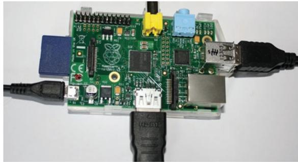
This image shows the Raspberry Pi's **GPIO (General Purpose Input Output)** connector. The Raspberry Pi operates at 5v DC and it is possible to connect components that do not draw a large current e.g. **LEDs (Light Emitting Diodes)** without using an interface board. However, you still need to ensure that you know the voltage required so that you do not cause damage to the Raspberry Pi.
