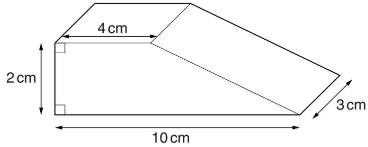
Draw full size the plan view, a front view and a side view of the door wedge.
