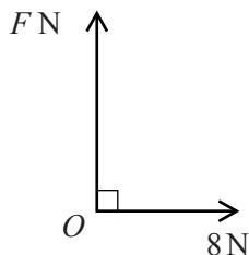
Two perpendicular forces of magnitudes  $F\text{ N}$  and  $8\text{ N}$  act at a point  $O$  (see diagram). Their resultant has magnitude  $17\text{ N}$ .
