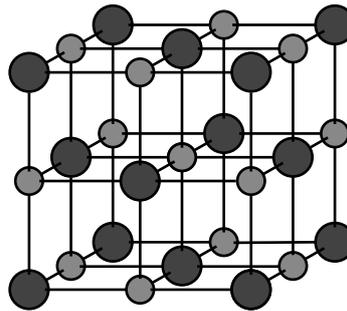
**Fig. 1:** cubic lattice structure of LiF
