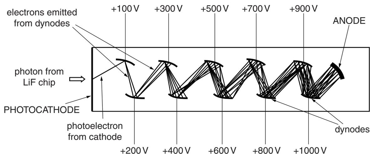
**Fig. 3:** schematic diagram of a photomultiplier tube
