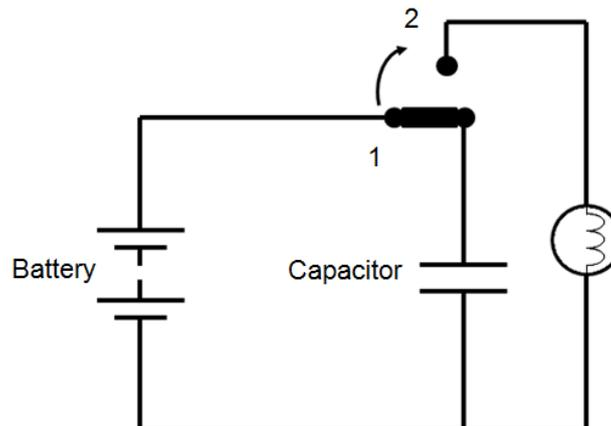
The lamp will glow for a time, and then dim till it goes out due to voltage (charge) in capacitor discharging.
