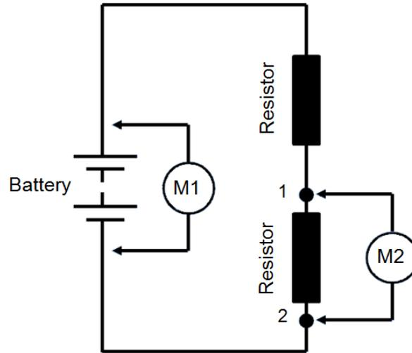
a) What quantity is meter M1 measuring – electromotive force (EMF) or potential difference (PD)?
