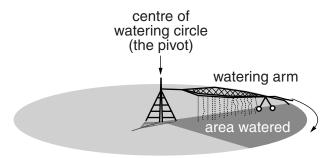
A long pipe on wheels pumps out water whilst rotating about the pivot. A circular area is watered with the pivot at its centre.
