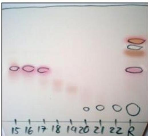
Figure 1 A chromatogram showing separated amino acids stained with ninhydrin.
