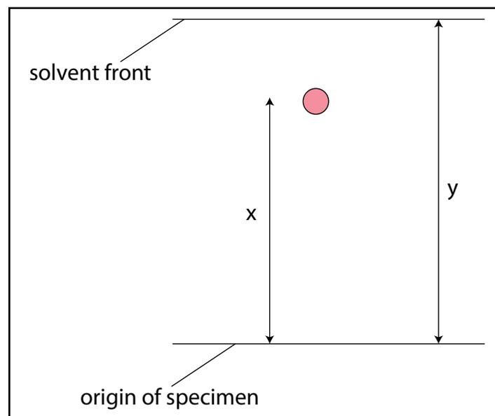
Figure 2 A diagram of a chromatogram indicating the measurement to take for the solvent front (y) and the measurement to take for distance travelled by sample (x).
