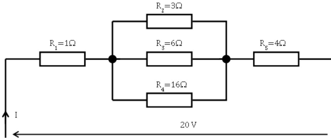
Activity 1 involves a circuit with series and parallel resistances, and an applied voltage. The problems can be solved by calculating overall circuit resistance and using Ohm's Law to calculate current. Learners will require some knowledge of series and parallel resistor combinations and Ohm's Law before attempting the problem.
