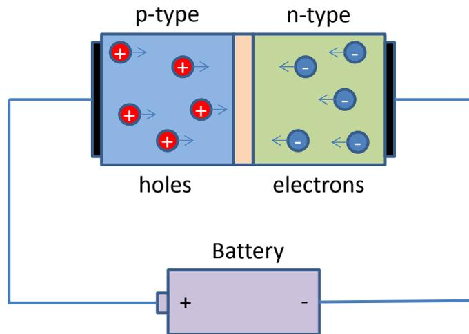
If a voltage is applied to the diode (n-type end positive and p-type end negative) positive electrons now move towards the p-type electrode and negative holes towards the n-type electrode. The diode is now **reverse biased** and the diode blocks the flow of current.
