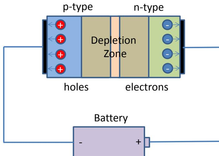
So – the diode conducts current in one direction and blocks the flow of current in the other direction. The positive terminal (p-type end) of the diode is called the **anode** and the negative terminal (n-type end) the **cathode**.
