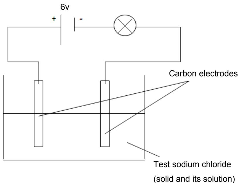
Dip carbon electrodes into some solid sodium chloride.
