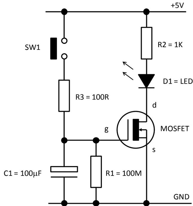
With SW1 closed, a voltage is applied to the gate terminal of the MOSFET and C1 also charges.
