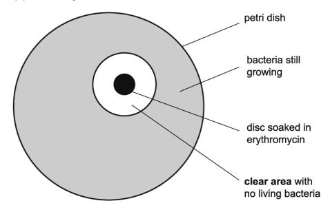
Use a ruler to measure the diameter of the clear area in mm.
