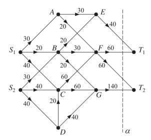
The diagram represents a system of pipes through which fluid can flow from two sources,  $S_1$  and  $S_2$ , to two sinks,  $T_1$  and  $T_2$ . It also shows a cut  $\alpha$ . The weights on the arcs show the capacities of the pipes in gallons per hour.
