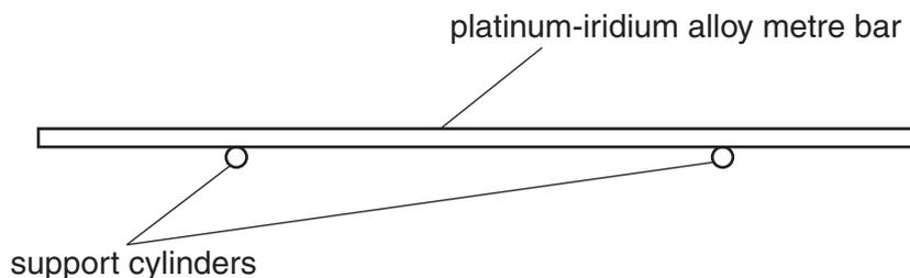
**Fig. 2** Arrangement for supporting the 1927 standard metre bar
