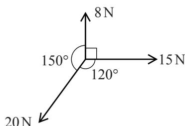
Three horizontal forces of magnitudes  $8\text{ N}$ ,  $15\text{ N}$  and  $20\text{ N}$  act at a point. The  $8\text{ N}$  and  $15\text{ N}$  forces are at right angles. The  $20\text{ N}$  force makes an angle of  $150^\circ$  with the  $8\text{ N}$  force and an angle of  $120^\circ$  with the  $15\text{ N}$  force (see diagram).
