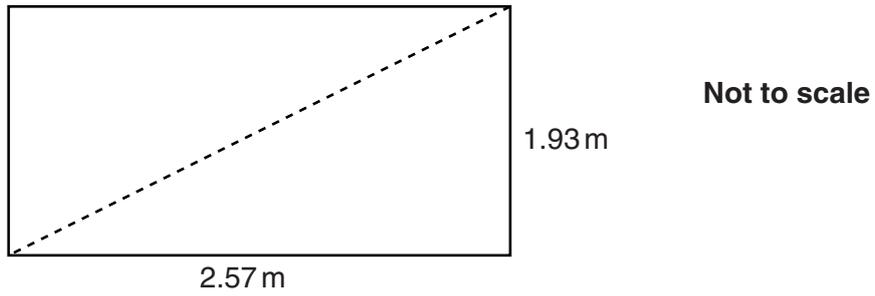
Dave checks that the base is a rectangle by measuring the diagonals.
