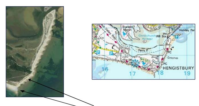
The aerial photograph above shows clearly that the groynes are trapping sediment, forming beaches. The beaches are wider on the south western side of the groynes. This is also shown at the largest groyne or breakwater at Hengistbury Head where the beach on the western side is almost three times as wide.
