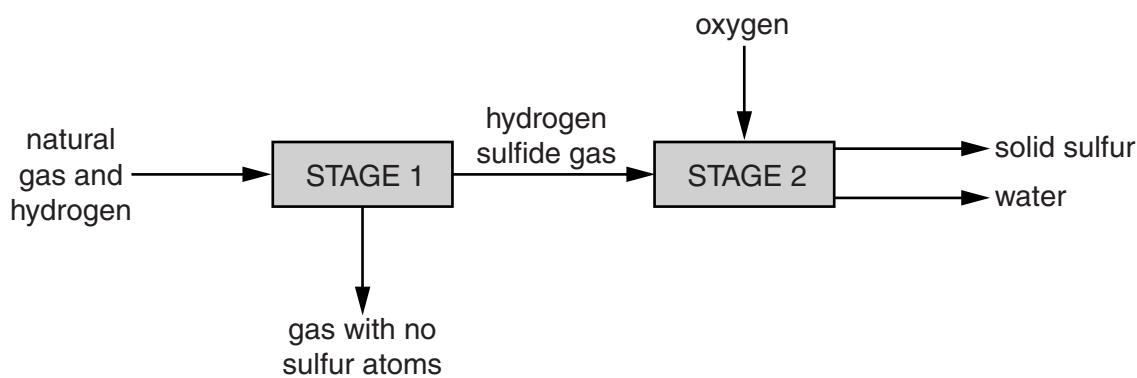
Stage 2 converts hydrogen sulfide into water and sulfur.
