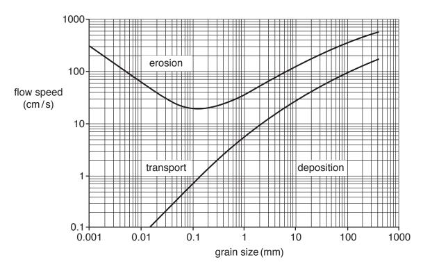
(i) State the minimum velocity required to transport a sediment size of 6 mm.
