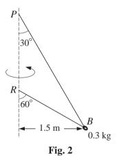
The lower part of the string is now attached to a point R, vertically below P. PB makes an angle  $30^{\circ}$  with the vertical and RB makes an angle  $60^{\circ}$  with the vertical. The bead B now moves in a horizontal circle of radius 1.5 m with constant speed v m s<sup>-1</sup> (see Fig. 2).
