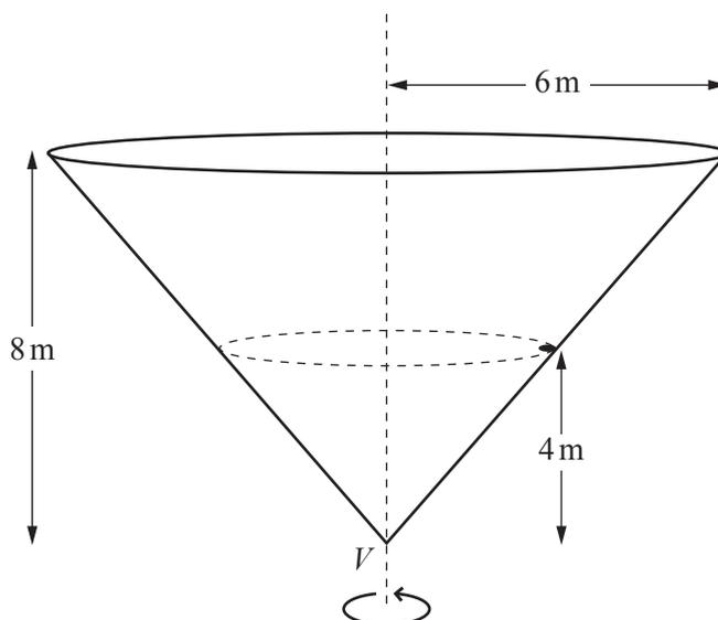
A conical shell has radius 6 m and height 8 m. The shell, with its vertex  $V$  downwards, is rotating about its vertical axis. A particle, of mass 0.4 kg, is in contact with the rough inner surface of the shell. The particle is 4 m above the level of  $V$  (see diagram). The particle and shell rotate with the same constant angular speed. The coefficient of friction between the particle and the shell is  $\mu$ .
