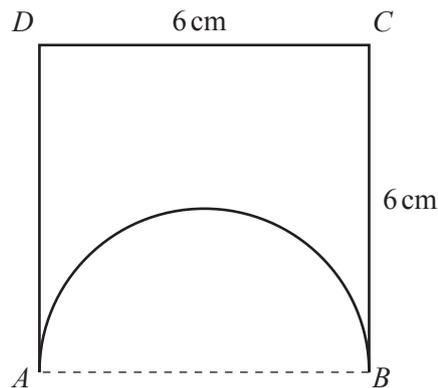
A uniform square lamina  $ABCD$  of side 6 cm has a semicircular piece, with  $AB$  as diameter, removed (see diagram).
