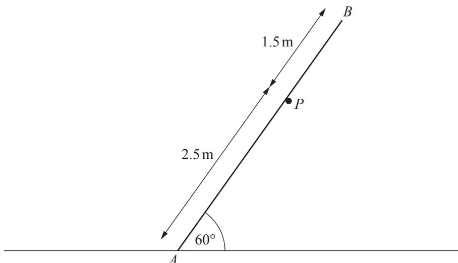
A uniform rod  $AB$ , of mass 3 kg and length 4 m, is in limiting equilibrium with  $A$  on rough horizontal ground. The rod is at an angle of  $60^\circ$  to the horizontal and is supported by a small smooth peg  $P$ , such that the distance  $AP$  is 2.5 m (see diagram). Find
