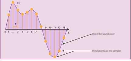
The number of samples taken per unit of time is called the **sample rate**. The higher the sample rate, the better the quality of the sound playback as the digital wave will follow the analogue sound wave pattern closely. However, the more samples that are taken, the more bits will be stored so the larger the file size will be. Sample rates are measured in Kilohertz (KHz). Typical rates are between 44.1 – 192KHz.
