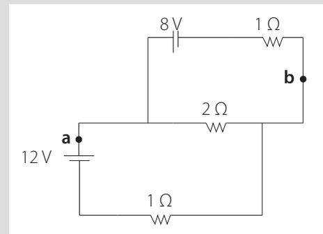
1. In the circuit above, find the current through the 2 ohm resistor and the potential difference between point a and b.
