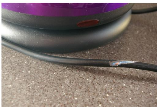
The insulation is damaged on the cable.
