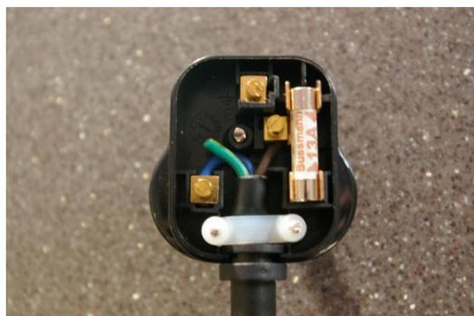
Type I appliances require an earth connection – the earth is missing (not connected) in the plug.
