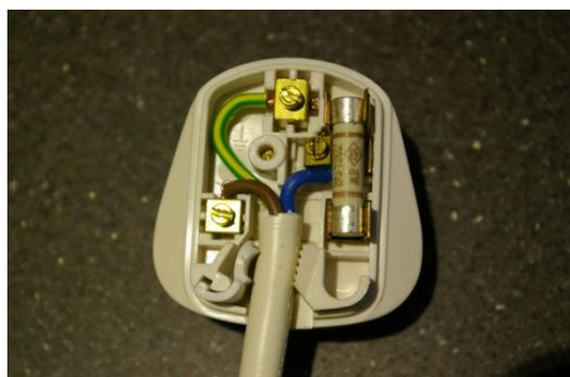
The live and neutral wires have been transposed.
