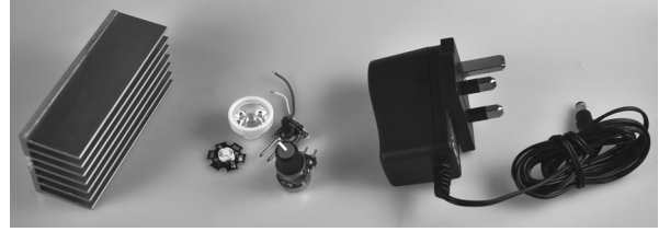
heat-sink, LED, lens, control circuitry, power supply
