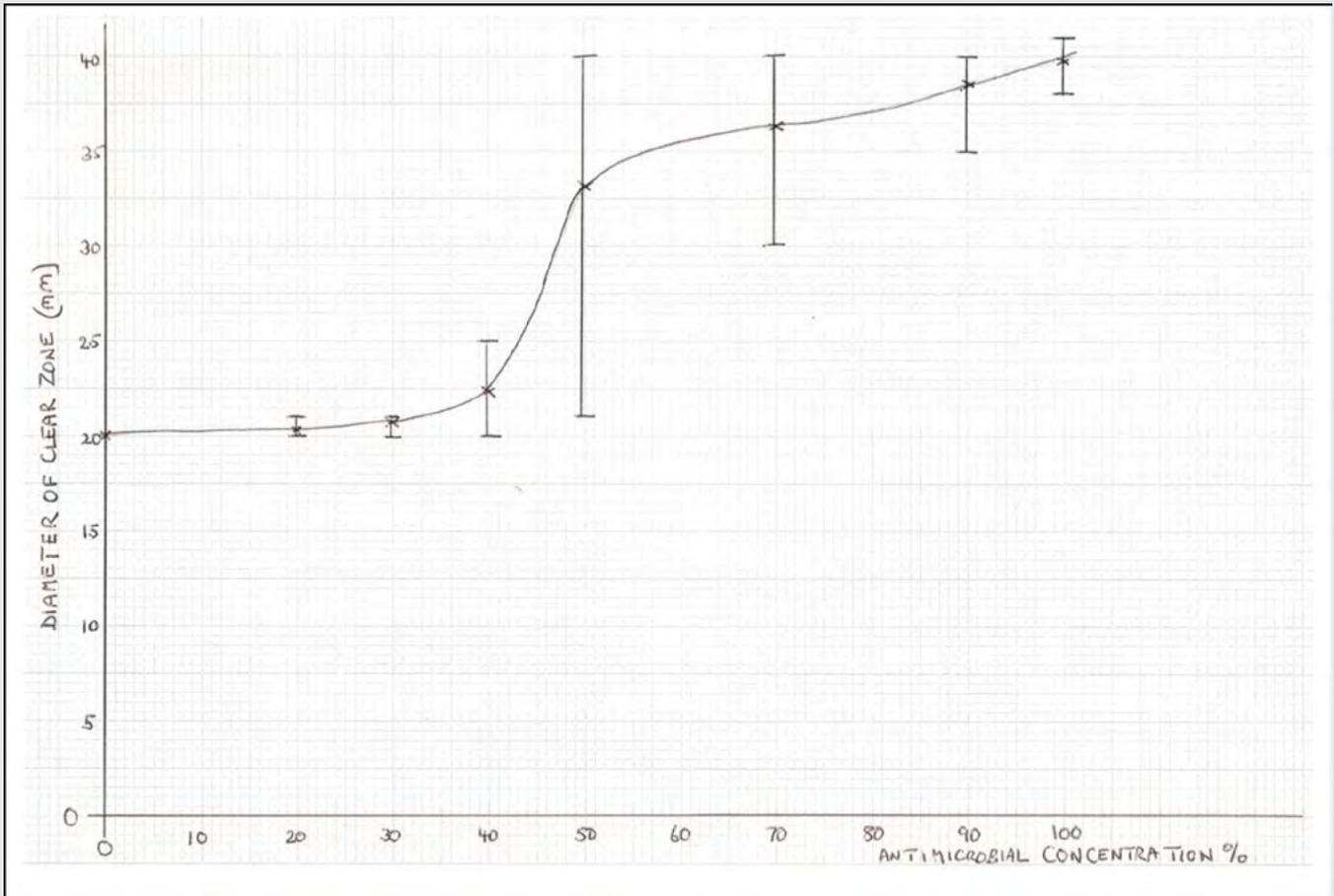
Within the concentration range of 0% - 40% the repeatability for the test is within 20mm to 25 mm giving a minimum accuracy of 20%. Within the concentration range of 70% to 100% the minimum accuracy was 25% however the accuracy between the 40% and 70% concentration the accuracy of the results dropped to 60%.
