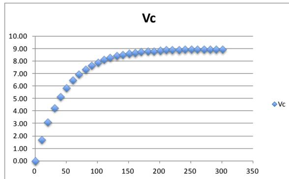
2. The time constant for the circuit is  $RC$  (learners will need to know that resistance is in kilohms and capacitance is in microfarads in order to calculate this). The time constant is 47 seconds.
