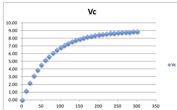
1. The shape of the graph is still an exponential – but in this case the capacitor takes longer to charge up.
