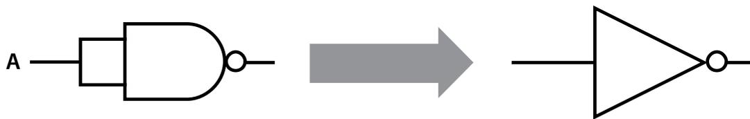
The logic is  $\overline{A \cdot A}$ , which, as we know from simplification, is  $\bar{A}$
