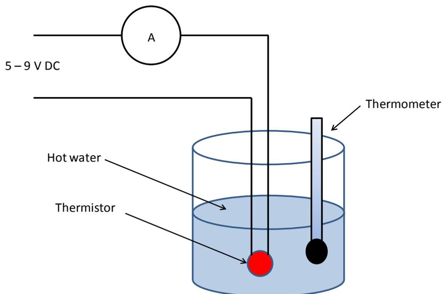
Learners should tabulate and plot their results from the experiment. In order to determine resistance of the device, learners could use Ohm's Law.
