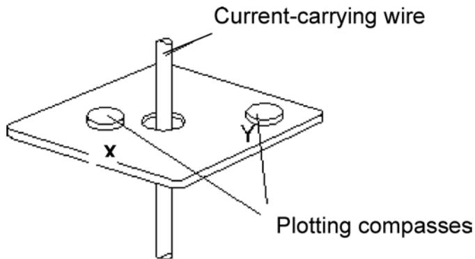
Compared to **Y**, the strength and direction shown on the compass, of the magnetic field at **X** is:
