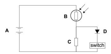
(i) Which component in the circuit is the LDR?
