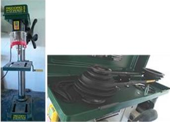
The pictures above show a pillar drill used in a home workshop. It has a pulley and belt drive system connecting the motor at the back of the machine to the chuck. Five ratios are available to give a range of chuck speeds to suit different drilling operations.
