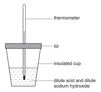
He uses the same volume and concentration of the acid and the sodium hydroxide every time.
