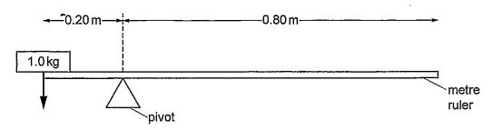
(a) Calculate the moment of the 1.0 kg mass about the pivot, in units of Nm.
