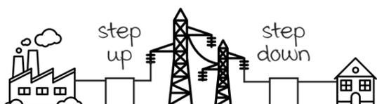
The National Grid uses step-up and step-down transformers to reduce the current and increase voltage in transmission lines.
