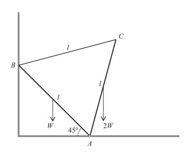
The uniform rods AB, of length l and weight W, and AC, of length l and weight 2W, are freely pivoted to a fixed point A. The rods are at rest in equilibrium in a vertical plane which is perpendicular to a smooth vertical wall. B rests against the wall and A is on a horizontal floor. AB is inclined at an angle of  $45^{\circ}$  to the horizontal. The ends B and C of the rods are joined by a light inextensible string of length l so that triangle ABC is equilateral (see diagram).
