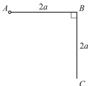
A compound pendulum consists of two uniform rods  $AB$  and  $BC$ , each of length  $2a$  and mass  $m$ . The rods are rigidly joined together so that  $AB$  is perpendicular to  $BC$ . The pendulum is freely hinged to a fixed point at  $A$ . The pendulum can rotate in a vertical plane about a smooth fixed horizontal axis through  $A$  (see diagram).
