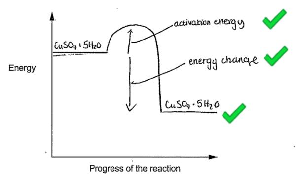
This response illustrates a correctly drawn and labelled reaction profile. The candidate's answer illustrates the comment that examiners only gave credit for correctly drawn single headed arrows, as is the correct convention for reaction profile diagrams.
