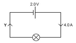
Write down the current flowing at point  ${\bf Y}$  in the circuit.
