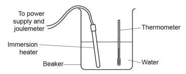
He heats up 1kg of water, using an immersion heater. He measures the temperature rise and calculates the specific heat capacity of the water.
