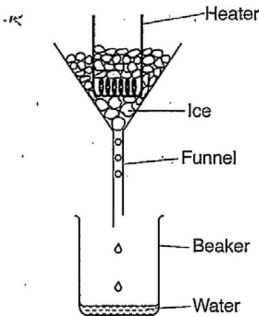
$$\text{latent heat} = \frac{\Delta \text{thermal energy}}{\text{mass}}$$
