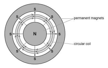
The direction of the magnetic field between the poles is shown as ------▶.
