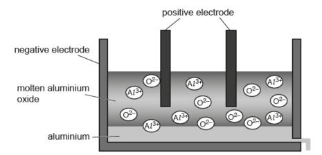
(a) The aluminium oxide must be molten in this process so that it conducts electricity.
