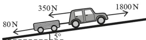
A car and a trailer are moving together along a straight road up a hill inclined at  $5^\circ$  to the horizontal. The car has a driving force of magnitude 1800 N and a resistance to motion of 350 N. The trailer has a resistance to motion of 80 N. A light rigid tow-bar parallel to the road joins the trailer to the car (see diagram). The mass of the car is 1250 kg and the mass of the trailer is 150 kg.
