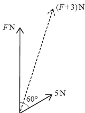
Two horizontal forces of magnitudes  $F \text{ N}$  and  $5 \text{ N}$  act on bearings  $000^\circ$  and  $060^\circ$  respectively. The resultant of these two forces has magnitude  $(F + 3) \text{ N}$ , as shown in the diagram.
