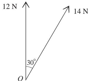
Two horizontal forces act at the point  $O$ . One force has magnitude 12 N and acts along a bearing of  $000^\circ$ . The other force has magnitude 14 N and acts along a bearing of  $030^\circ$  (see diagram).
