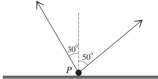
A particle  $P$  of weight  $30\text{ N}$  rests on a horizontal plane.  $P$  is attached to two light strings making angles of  $30^\circ$  and  $50^\circ$  with the upward vertical, as shown in the diagram. The tension in each string is  $15\text{ N}$ , and the particle is in limiting equilibrium. Find
