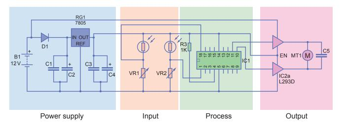
Fig. 8 – Microcontroller circuit
