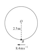
A smooth wire is shaped into a circle of radius 2.5 m which is fixed in a vertical plane with its centre at a point *O*. A small bead *B* is threaded onto the wire. *B* is held with *OB* vertical and is then projected horizontally with an initial speed of  $8.4 \text{ m s}^{-1}$  (see diagram).
