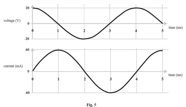
(i) Use the graphs in Fig. 5 to find the frequency of the current in the inductor.
