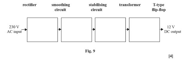
This question was one of the most successfully attempted on the paper, and would have been more so were it not for a sizeable group that incorrectly interchanged the smoothing circuit and the stabilising circuit.
