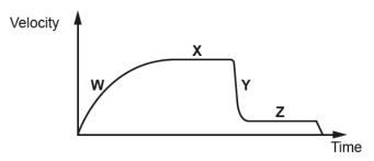
Which parts of the graph show balanced forces on the skydiver?
