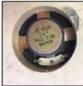
Glue speaker into speaker drill hole
