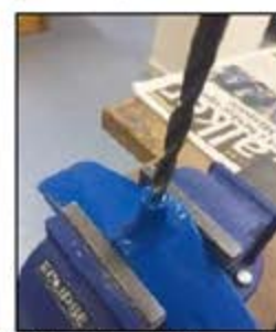
Drill hole for delivery tube
