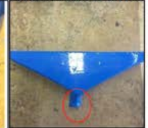
However the first attempt of funnel came out wonky and the plastic was shriveled at the tube
