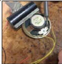
Solder speaker to wires
