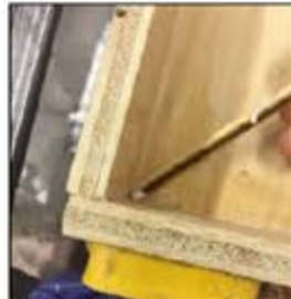
Get rid of glue around edges and inside of box
