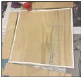
Assemble box using wood glue
