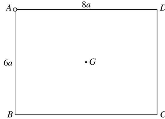
The diagram shows a uniform rectangular lamina  $ABCD$  with  $AB = 6a$ ,  $AD = 8a$  and centre  $G$ . The mass of the lamina is  $m$ . The lamina rotates freely in a vertical plane about a fixed horizontal axis passing through  $A$  and perpendicular to the lamina.
